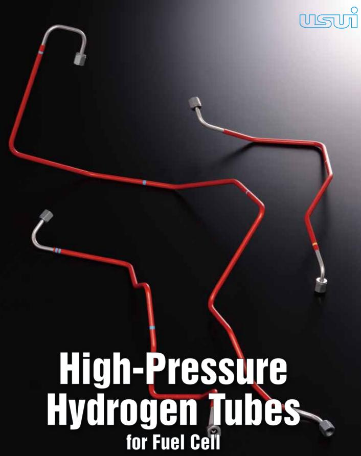
This is a stainless tube which is used to deliver hydrogen gas from a high pressure hydrogen gas tank of a Fuel Cell. The metal sealing design, combined with a tightening nut improves assembly performance while maintaining high pressure sealing.
